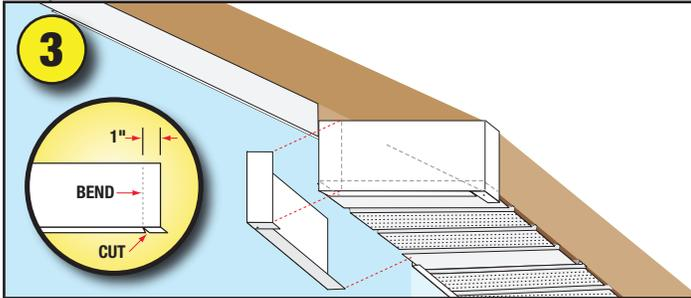
**3. FASCIA TRIM** - Beginning at corners, cut and bend to form box. With box in position, pre-drill (align with soffit grooves) and nail through bottom lip of fascia trim every 36 inches along bottom edge of fascia board. Never 'face nail' fascia. Do not drive nails tight - fascia must be 'hung', to allow expansion and help prevent distortion.
