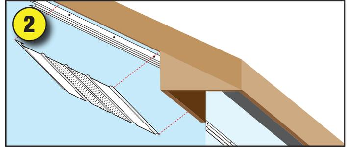
**2. GABLE END SOFFIT PANELS** - Start at the base of the gable end and work up to the peak from each side, as far as full panels will fit. Slide panels into channel and secure to under edge of fascia board. It may be necessary to cut a panel, bend to match peak angle and rebend edges to make interlocking jointings. Slide peak panel into position and nail.
