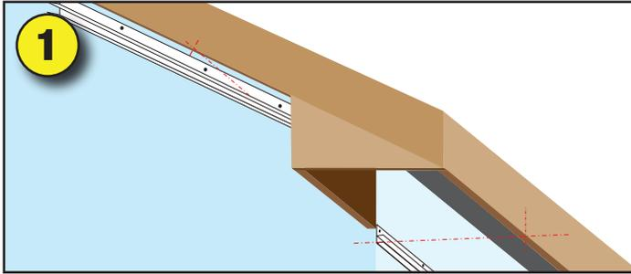
**1. FRIEZE RUNNER** - Bottom edge of runner channel must be level and aligned with the bottom surface of the fascia board. Using nailing flange of channel, nail and install along the entire length of the wall surfaces and up to gable peak on side wall
