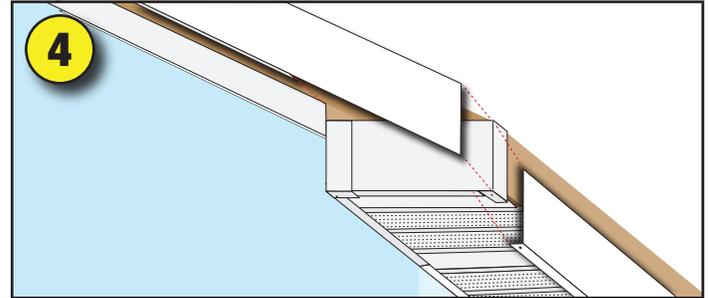
**4. FINISH TRIM** - Allow at least 1 inch overlap of fascia where lengths meet. Cover balance of gable end with fascia trim and cut to make overlap joint at peak. Use drip edge or trim coil to cover and finish top edge of fascia trim.
